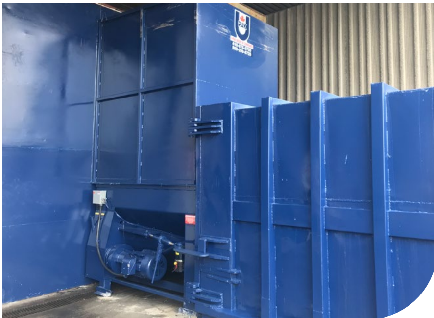
A cardboard compactor at our Hamilton Mail Processing Plant helps to free up operational space and divert cardboard for recycling.
